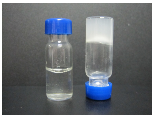
Fig. 1. The C/GP formulation at room temperature (left) and at 37°C (right)
